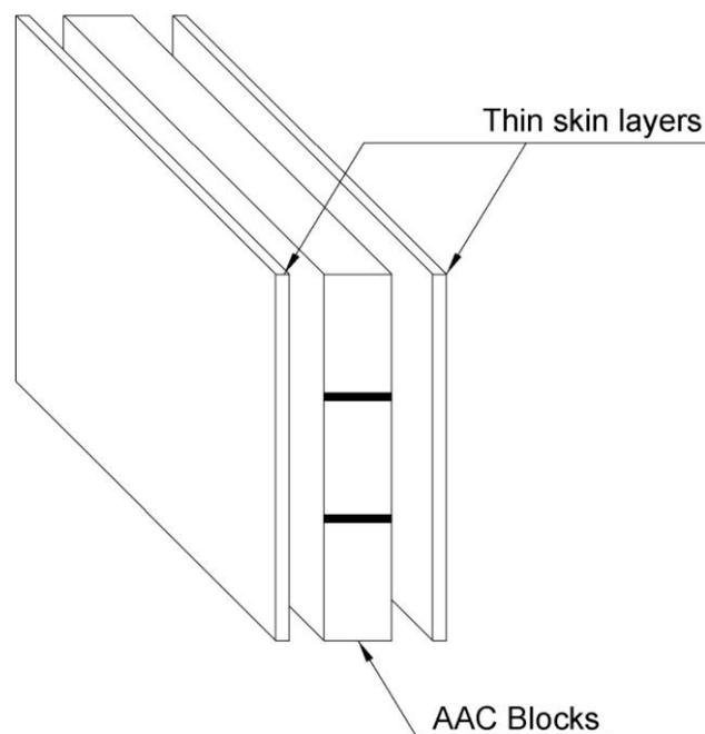
Figure 1.1: Ferrocement sandwich panel composed of two skin layers and AAC blocks
