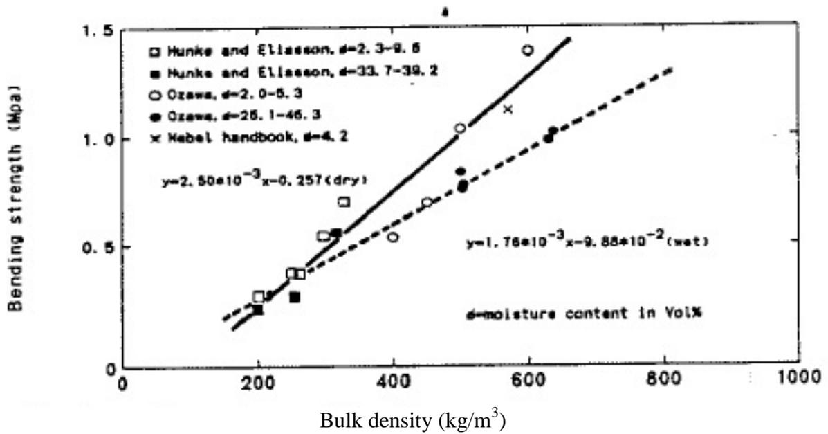
2.1b) Dependence of bending strength on bulk density (Tada, 1986)
