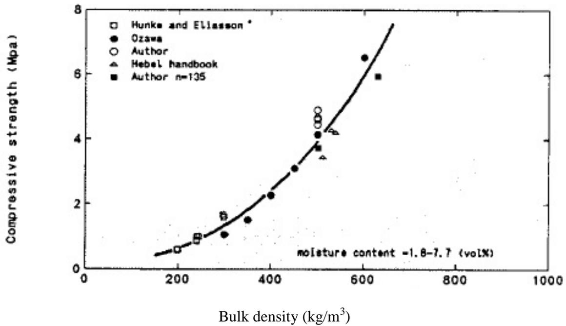
2.1c) Dependence of compressive strength on bulk density (Tada, 1986)
