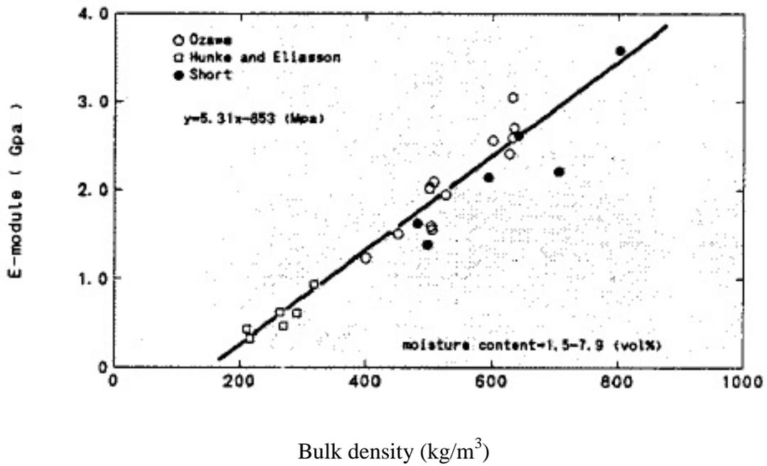
2.1a) Dependence of E-module on bulk density (Tada, 1986)
