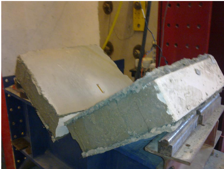
Figure 5.6: Typical failure pattern of specimen B1
