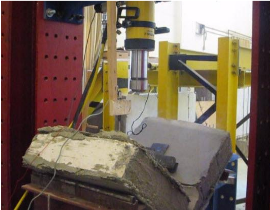
5.9a) Typical failure pattern
